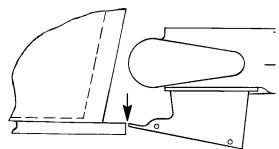
Fasten outboard to the transom at this height. Refer to the Outboard Operation and Maintenance Manual for instructions on securing outboard to the transom.
