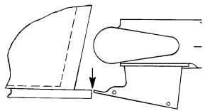
Fasten outboard to the transom at this height. Refer to the Outboard Operation and Maintenance
