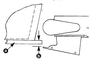
4. Raise The outboard up on the transom the distance measured in Step 3. Use a straight edge and recheck the mounting height. The top edge of the water intake housing should be in line with the bottom of the boat as shown.
